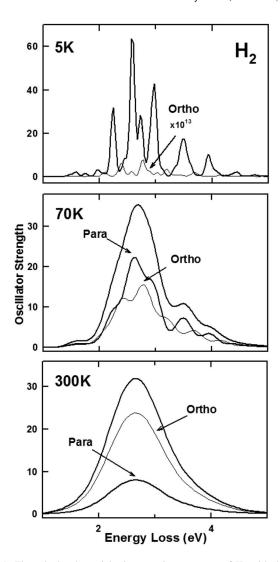
FIG. 4. The calculated quasielastic scattering spectrum of  $\rm H_2$  with decomposition into the contributions from ortho and para nuclear spin isomers at temperatures of 5, 70, and 300 K. Convolution with Gaussians of 50 meV FWHM was performed in order to show expected results from possible high resolution experiments.
