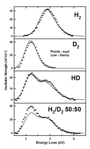
FIG. 1. The experimental quasielastic scattering spectra (Ref. 4) of  $H_2$ ,  $D_2$ , HD, and a 50:50 mixture of  $H_2$  and  $D_2$  (circles and error bars) compared to predictions of the present theory (solid line). The computed cross sections are absolute. The intensity scales for the experimental data were established by using the  $K^2S(0,K)$  sum rule to normalize the experimentally determined relative intensities.
