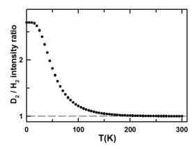
FIG. 3. The temperature dependence of the ratio of the intensity of quasielastic scattering from  $D_2$  relative to that for  $H_2$  in an equimolar mixture, at equilibrium, given by Eq. (13). The input parameters used in the calculation are listed in Table I and were taken from Refs. 31 and 32. The variation is related to the temperature dependence of the ortho-para equilibrium, and the difference in the ortho and para contributions to the rotational fine structure.
