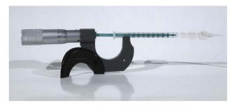
Figure 2. Portable nano-injector for 1 mL syringes, built from a micrometer gauge.
